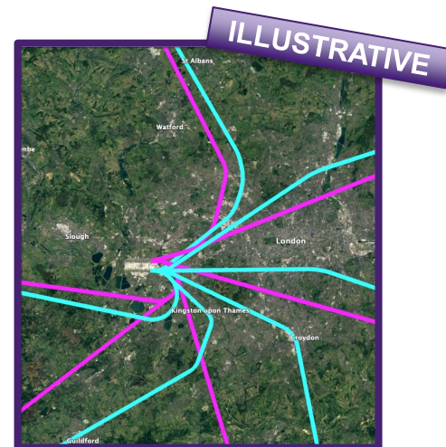
Example of how we could design different flight paths to keep routes from the two runways separate
