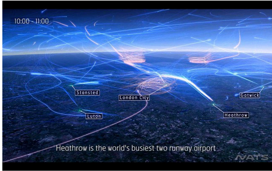
Heathrow's four holding stacks, or 'waiting rooms' for arriving aircraft. Source: NATS Press Office
