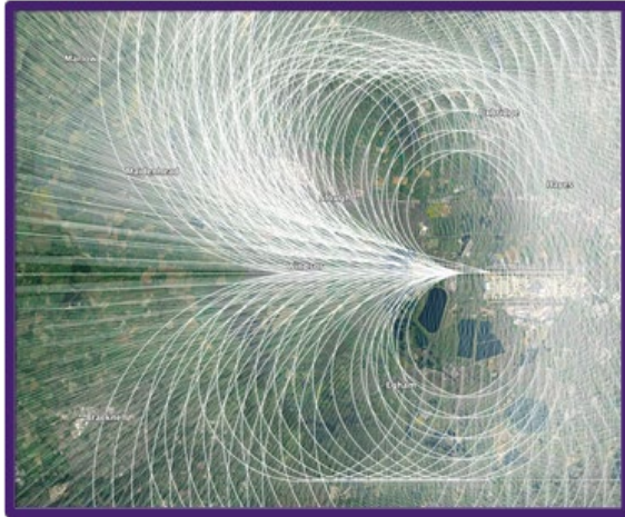
Sample of 'flooded' notional tracks for westerly departures from the northern runway – known as "27R departures"
