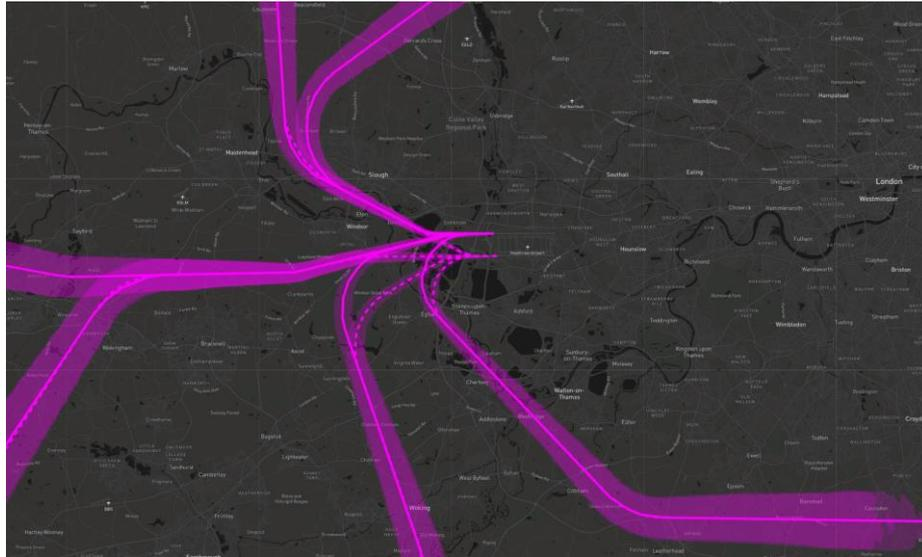
Figure 37: Illustration of Runway 27L Option F and Runway 27R Option F, routes that converge after departure
