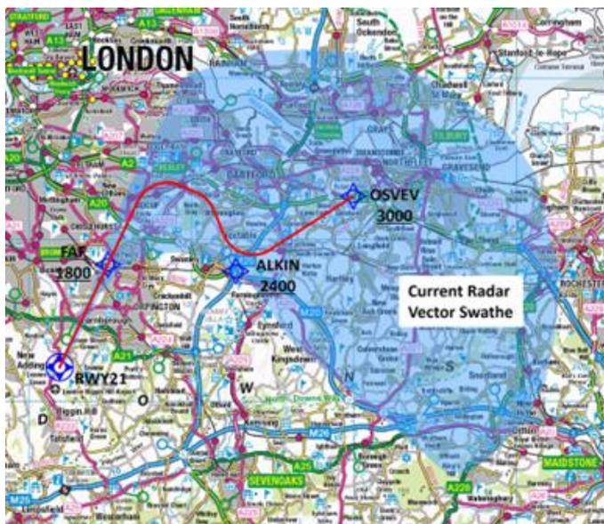
Satellite navigation available from Approach Transition – aircraft navigates into procedure from transition at OSVEV.
