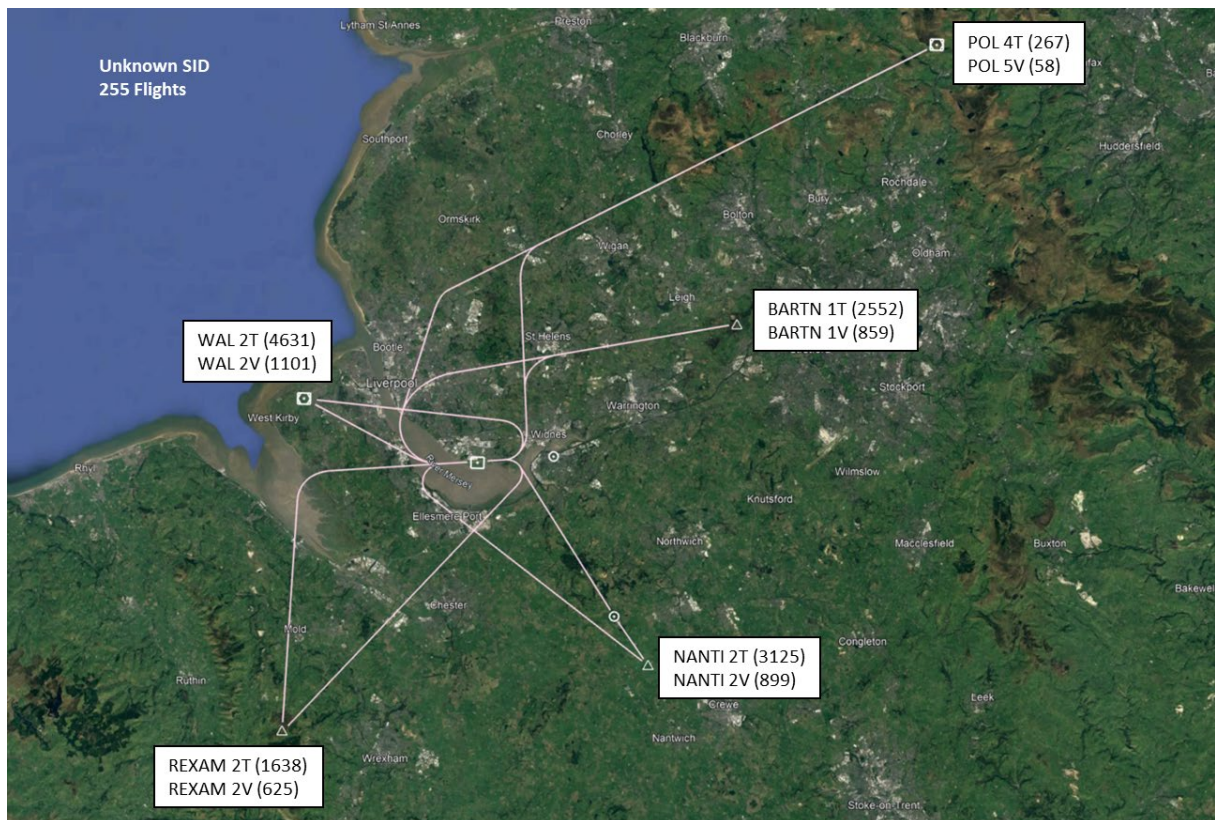
Figure 6: Google Earth map showing the SIDs departing LJLA. The SID's end letter determine which runway the SID relates to- a T for runway 27 or a V for runway 09.
