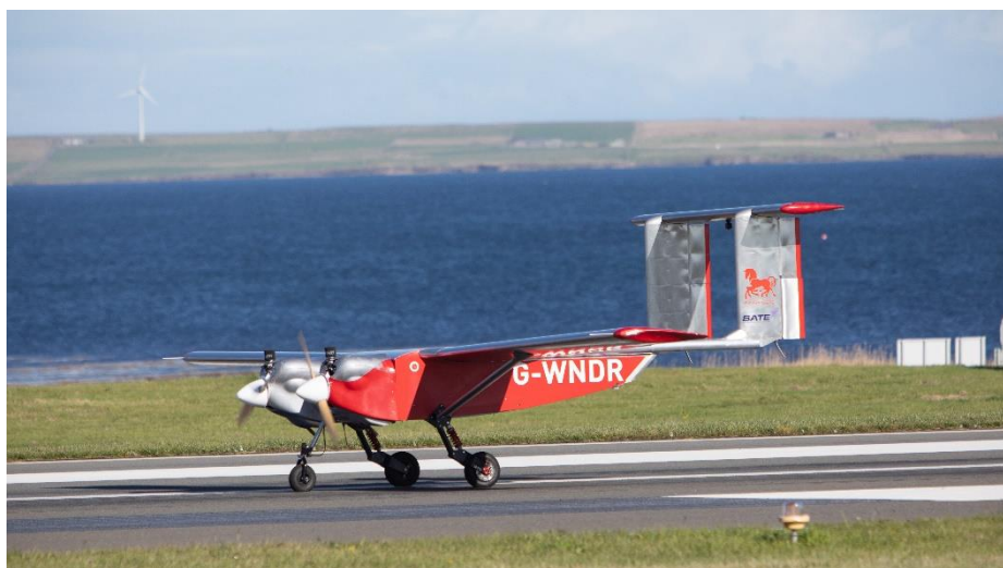
Figure 1 ULTRA UAS has been developed for robustness and redundancy of its flight critical systems (Photo credit to Colin Keldie at EMEC)
