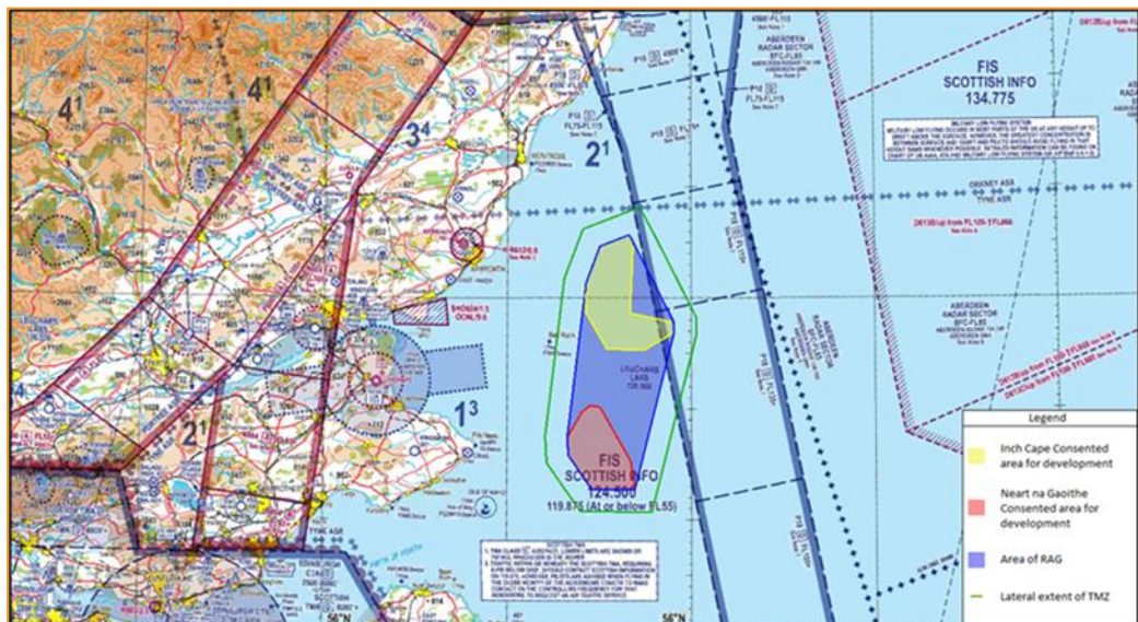
Figure 22 - NNG and IC TMZ Area (Circa 2015) Reproduced from CAA digital map data © Crown copyright 2015. UK AIP ENR.
