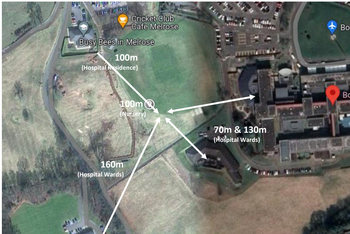
Figure 8 - The closest buildings and sensitive noise receptors to the Borders General Hospital TOLP
