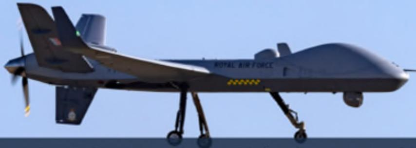
**Protector Stats:** Protector has a 79 ft wingspan and is 38 ft long. It is powered by a single TPE 331-10 turbo-prop engine and will be operated by fully qualified RAF crews
