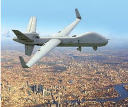
Protector has a 79FT wingspan and is 38FT long. It is powered by a single TPE 331-10 turbo-prop engine and will be operated by fully qualified RAF pilots.
