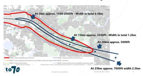
Airbus A320 – 60 dB LAmax contour vs Overflight Metric
