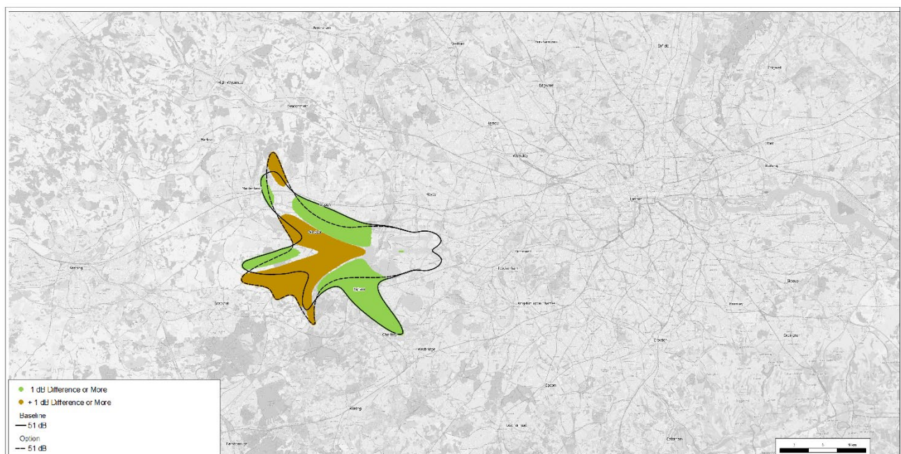
Figure 4: Change in noise exposure for Runway 27L Departure Option A 14 within the Partial LOAEL of at least 1dB compared to the baseline
