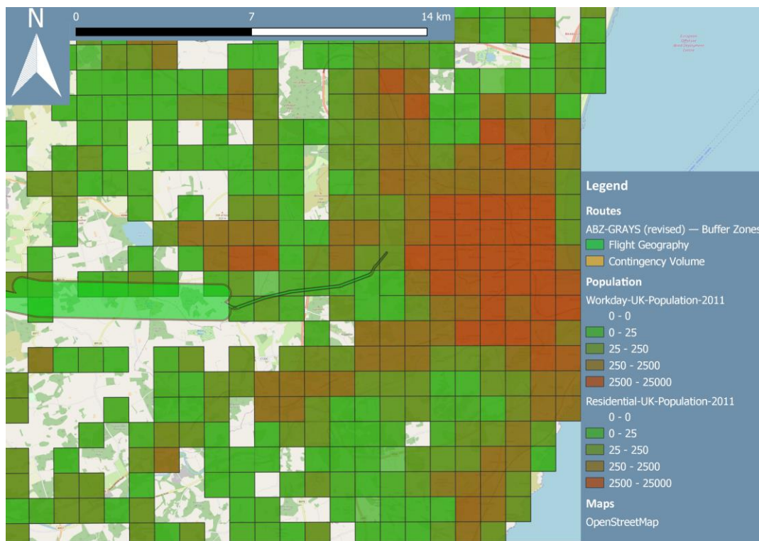
Figure 9 - Population density map with flight routes overlaid – Aberdeen TOLP – Dobbies Garden Centre
