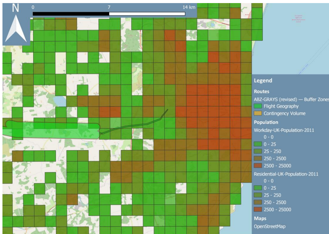
Figure 3 - Population density map with flight routes overlaid – Aberdeen TOLP – Dobbies Garden Centre
