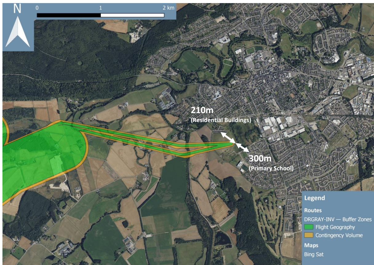
Figure 11 - The closest buildings and sensitive noise receptors to the Dr Grays TOLP
