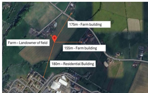
Figure 5: Crosshouse hospital TOLP, Option 2 TOLP and identified noise receptors and distance from TOLP (no information on how they will approach the TOLP is provided)
