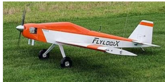
The Flylogix FX2, c. 50kg, wingspan 3.2m, flight duration c. 5-6hrs
