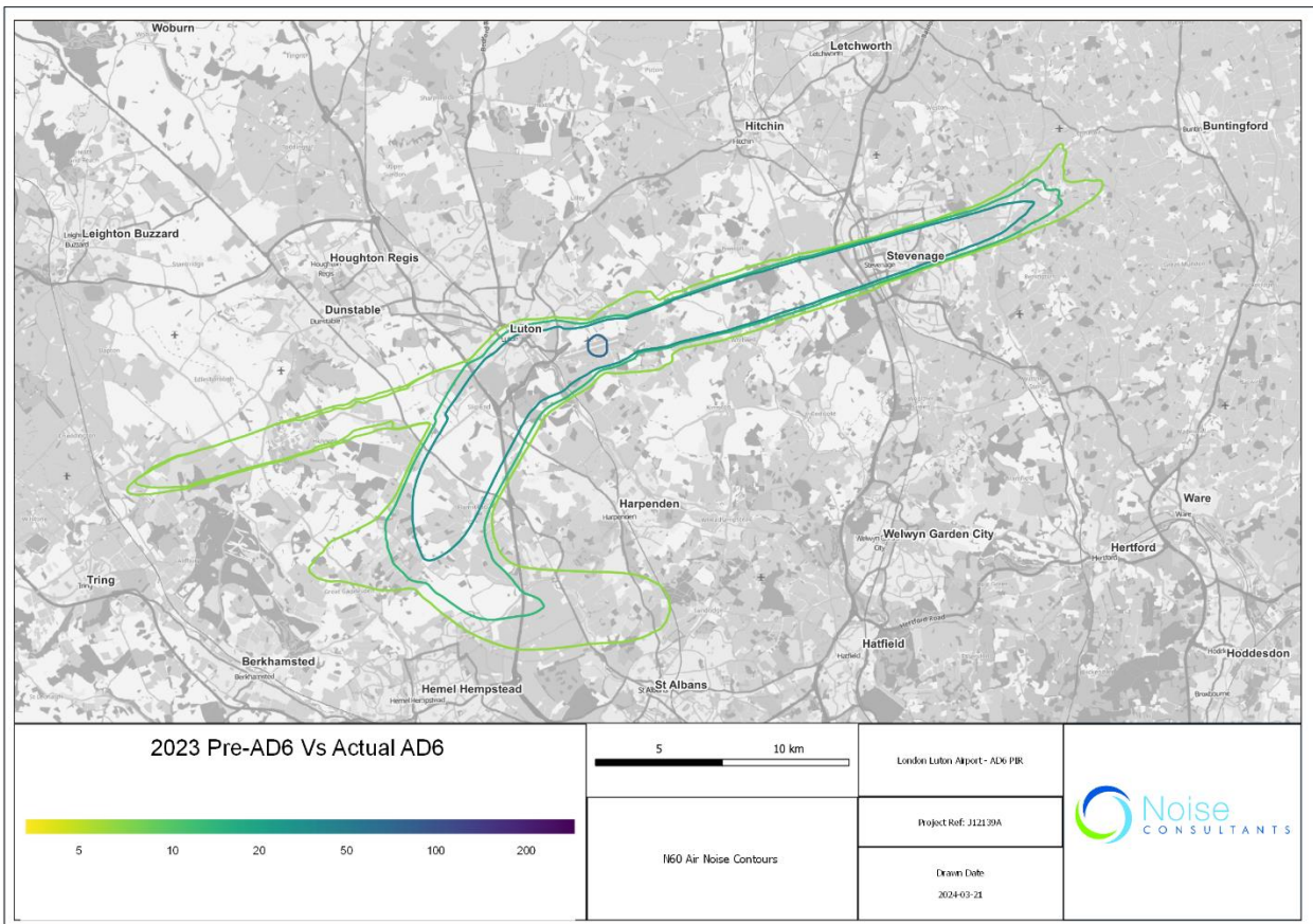
Figure 45 - N60 rate contours of the “2023 Without AD6” scenario overlaid with the contours of “2023 Actual”
