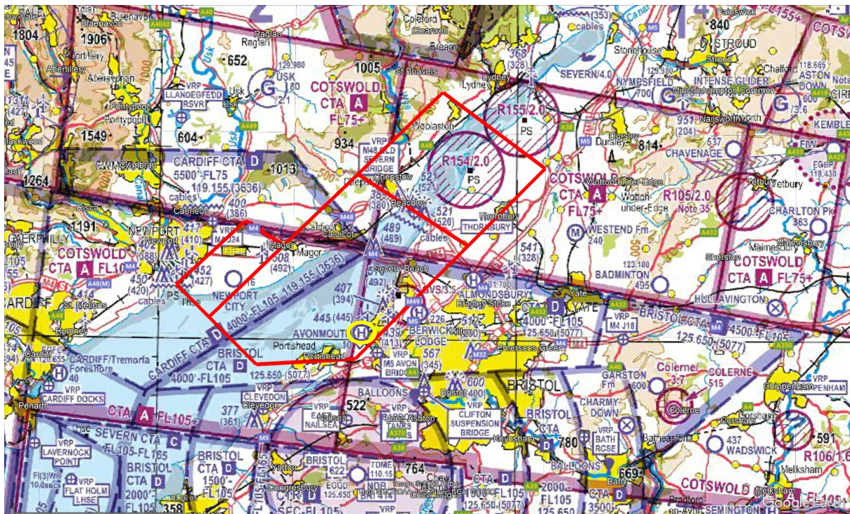
Figure 4: Current airspace displayed on a 1:500k VFR chart (March 2024). Proposed TRA and TMZ outlined in red. Avonmouth Helipad circled yellow.
