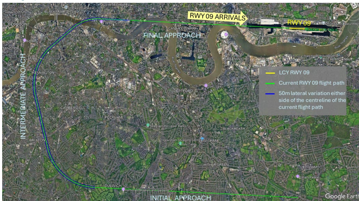
Figure 5: Initial/Intermediate Approach RWY09 Option 1 [IA09_Option 1] permits up to 50m lateral variation (shown in blue) from the centre line of the current flight path (shown in green). [Google Earth, 2025].
