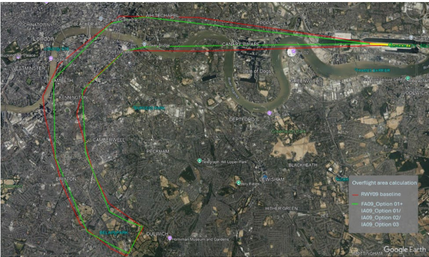
Figure 19: Overflight calculation for RWY09. The overflight area (or 'cone of overflight') for the baseline ('do nothing') option is shown in red, and the RNP AR approach options are shown in green. [Google Earth, 2025].
