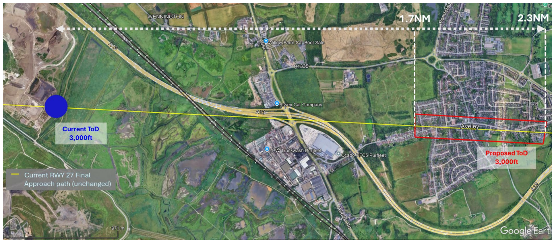
Figure 13: Final Approach RWY27 Option 2 [FA27_Option 2]. Detailed plan view - current ToD is shown in blue, proposed ToD is shown in red. [Google Earth, 2025].
