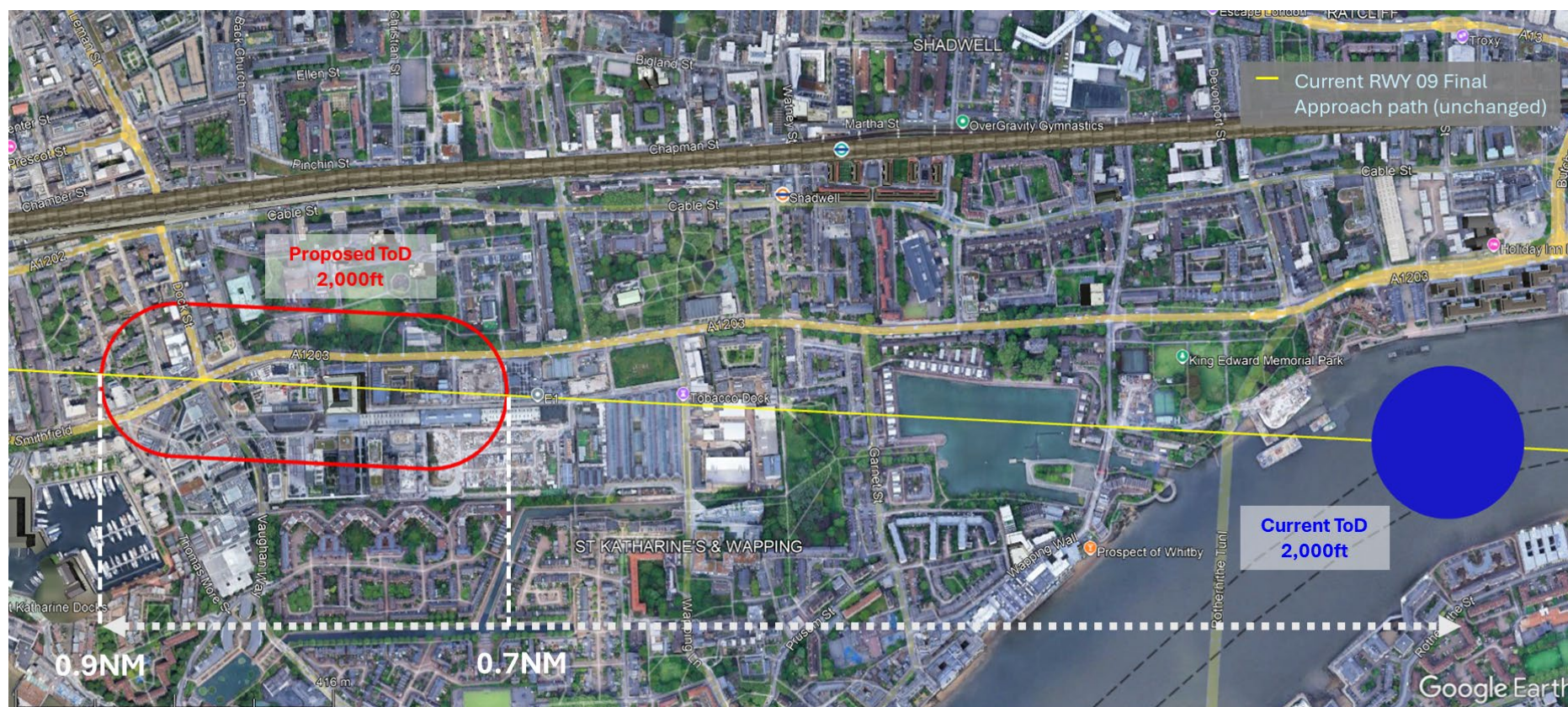
Figure 9: Final Approach RWY09 Option 1 [FA09_Option 1]. Detailed plan view - current ToD is shown in blue, proposed ToD is shown in red. [Google Earth, 2025].
