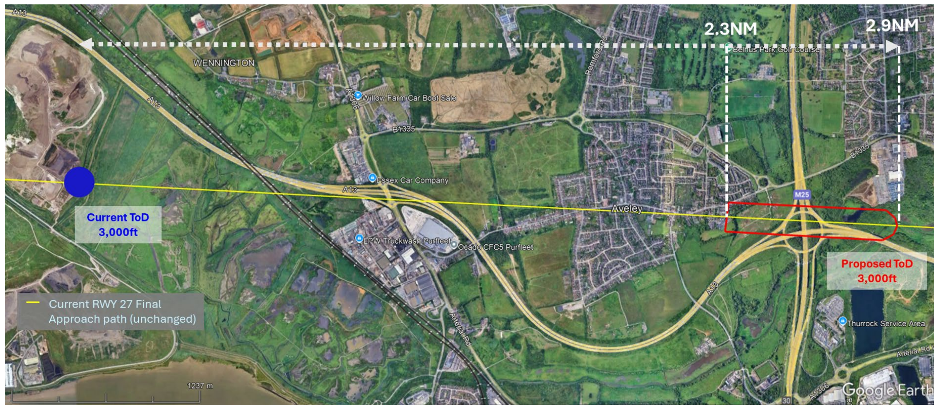
Figure 15: Final Approach RWY27 Option 3 [FA27_Option 3]. Detailed plan view - current ToD is shown in blue, proposed ToD is shown in red. [Google Earth, 2025].
