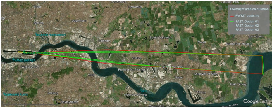
Figure 20: Overflight calculation for RWY27. The overflight area (or 'cone' of overflight) for the baseline ('do nothing') option is shown in red, and the RNP AR approach options are shown in green. [Google Earth, 2025].
