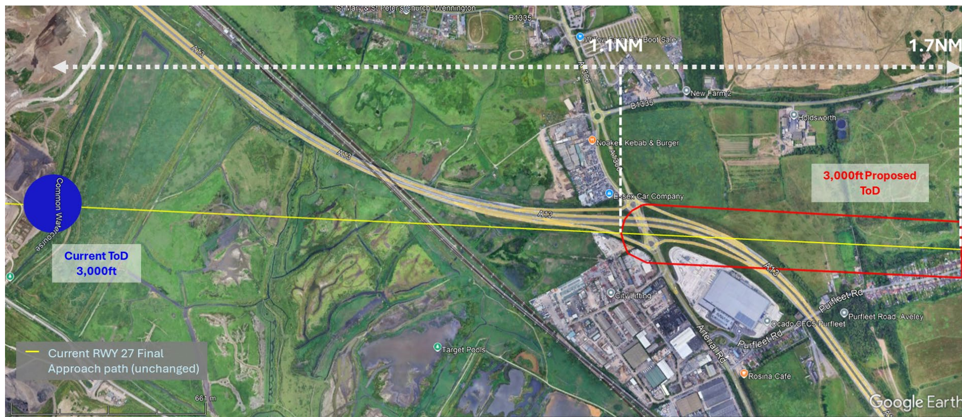
Figure 11: Final Approach RWY27 Option 1 [FA27_Option 1]. Detailed plan view - current ToD is shown in blue, proposed ToD is shown in red. [Google Earth, 2025].
