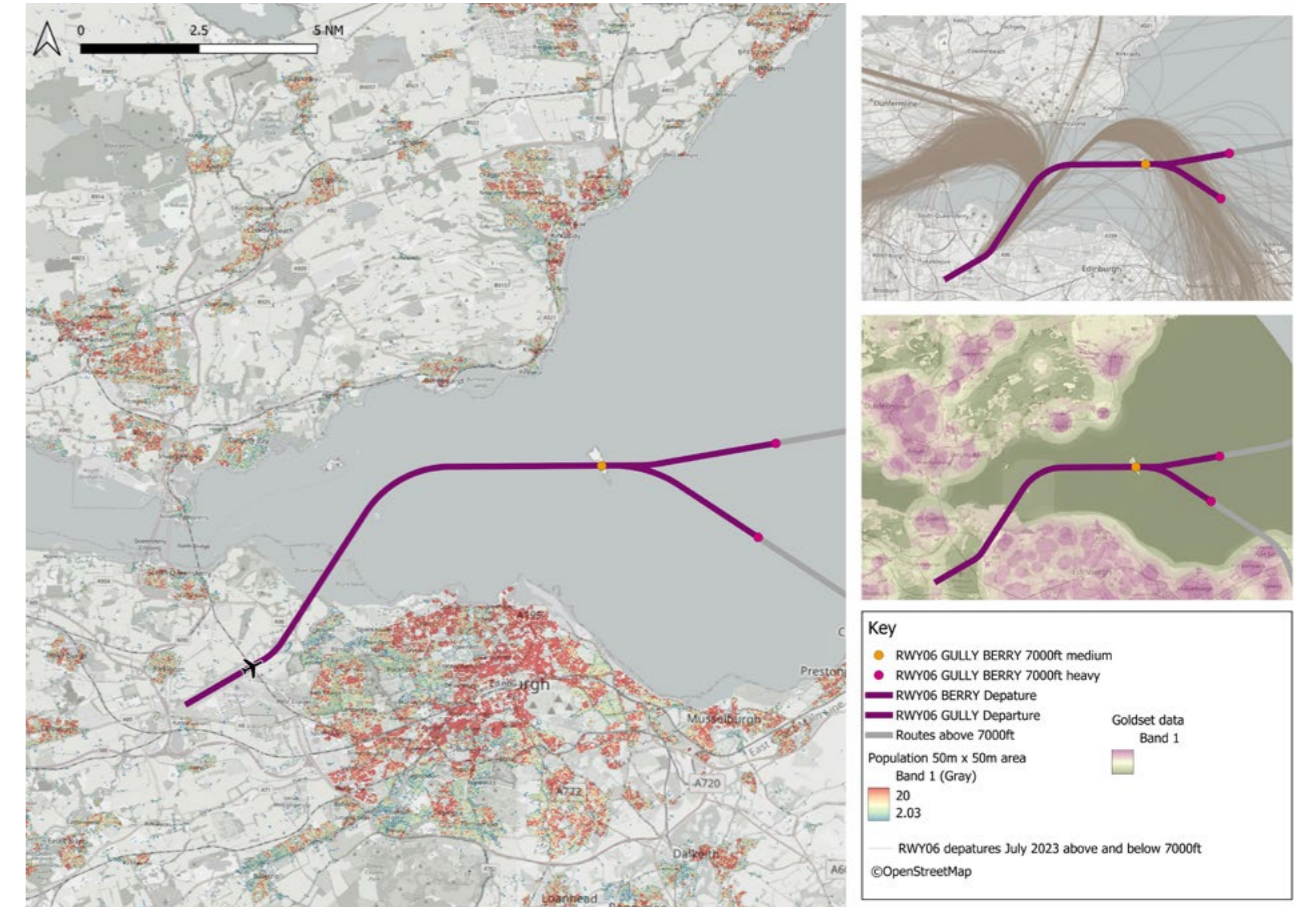
Figure 28: Design for runway 06 eastbound (GULLY and BERRY) overlaid population, today's tracks and GoldSET data.
