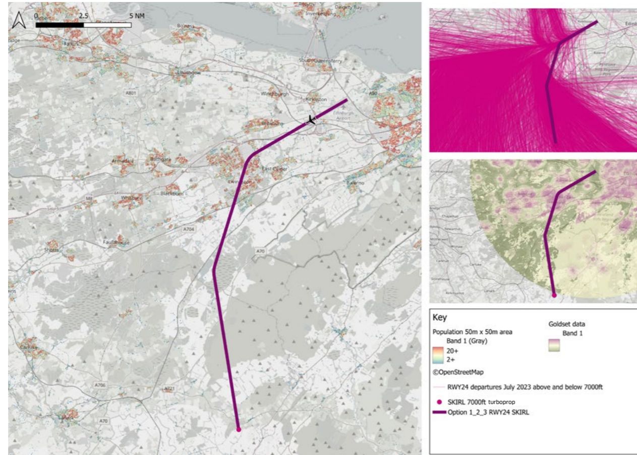
Figure 24: Design for runway 24 west/southbound turboprop only (SKIRL) overlaid population, today's tracks and GoldSET.
