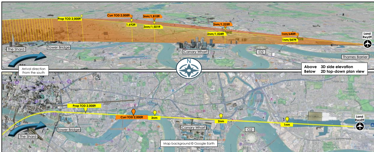
Figure 7 Final Approach diagram: Runway 09 differences in approach slope from 2,000ft, Current (Curr) 5.5° vs. Proposed (Prop) 4.49° and altitudes at 1nm intervals
