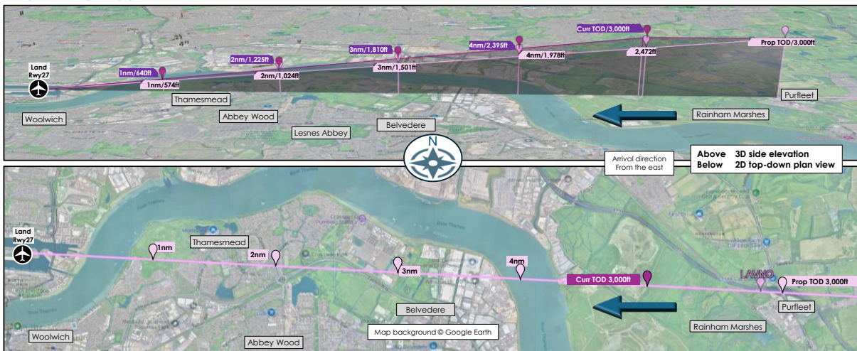
Figure 8 Final Approach diagram: Runway 27 differences in approach slope from 3,000ft, Current (Curr) 5.5° vs. Proposed (Prop) 4.49° and altitudes at 1nm intervals
