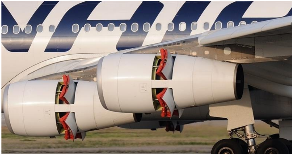
Figure 8 - Pivoting-door thrust reversal on an A340-300
